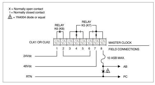
Figure B-5 Standard Electric Time AR-2A Two-Wired, Dual Voltage
